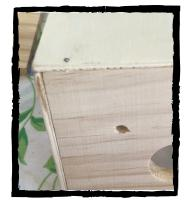
3. Now you'll nail down the other bottom piece of the birdhouse. Take the other smaller thin piece and make sure it overlaps a bit with the other bottom piece for a "tighter" seal. Nail this piece to the front and back of the birdhouse like you did before.
